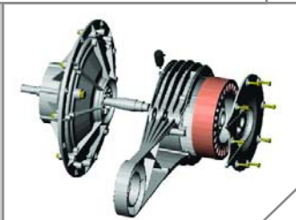
INTEGRATED MOTOR AND GEAR BOX
