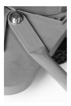
Fit the lower section of the handle over the handle posts on either side of the mower. Then place the washer over the post, insert the cotter pin and bend its ends back over the post as shown in above left photo. Continue assembly of the middle and top sections of the handle using the handle bolts and wing nuts as shown in above right photo.
