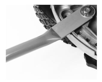
Fit the lower section of the handle over the handle posts on either side of the mower. Then place the washer over the post, insert the cotter pin and bend its ends back over the post as shown in above left photo. Continue assembly of the middle and top sections of the handle using the handle bolts and wing nuts as shown in above right photo.
