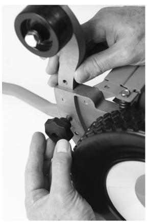
The cutting height of the CLASSIC may be adjusted from approximately 1.5 inch up to approximately 3.5 inches. Actual height may vary according to the density of the turf. Adjust the mower to the desired height first by rocking the handle forward so that it is sitting on the ground and the mower is upside down. The black height adjustment knobs are on the right and left of the mower body.
